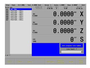
MILLPWR<sup>G2</sup> will automatically pause at points that require action to be taken (e.g., change tools). After each task has been completed, press the **G0** key.
