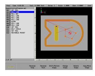
Machining a part in PGM mode will show the soft keys to easily select between 2D Line, 3D Line and 3D Solid without having to open the View Setup dialogue.
