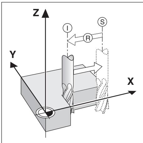
The position of the tool at any given moment is called the Actual Position **I**, while the position that the tool is to move to is called the Nominal Position **S**. The distance from the nominal position to the actual position is called the Distance-To-Go **R**.
