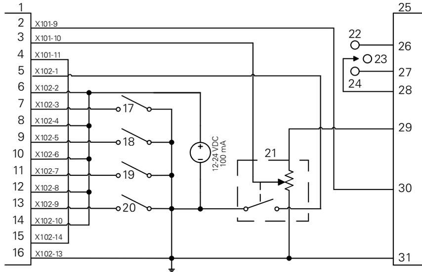
Example of gear detection and switching to manual spindle speed control
