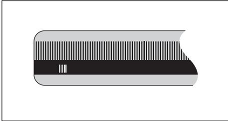
Encoders that have one or more marks on fixed intervals have to re-establish the datums correctly. It is necessary to use the same exact reference mark, during the Reference Mark Evaluation routine, that was used when the datum was first established.
