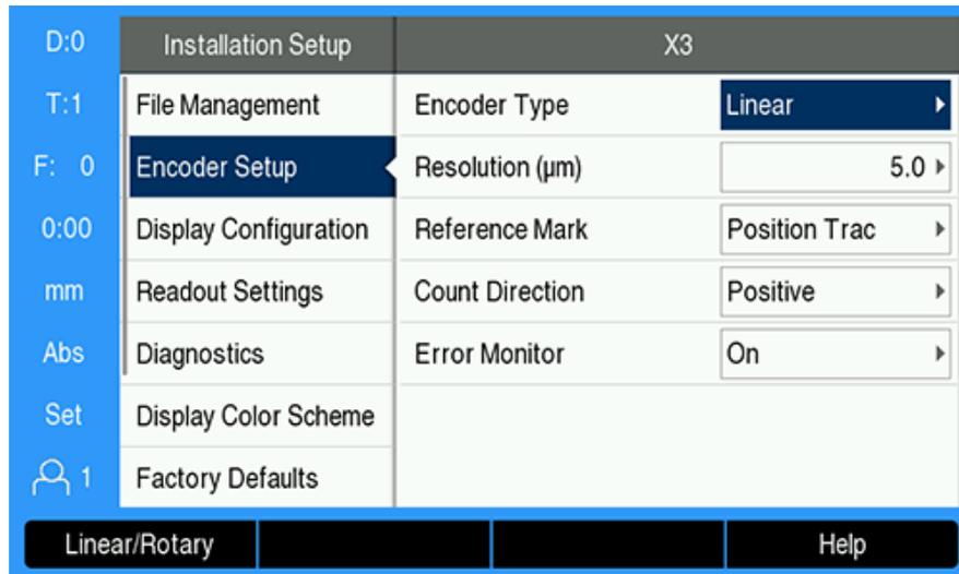
To set the **EDM Axis Encoder Type** to **Linear**:
