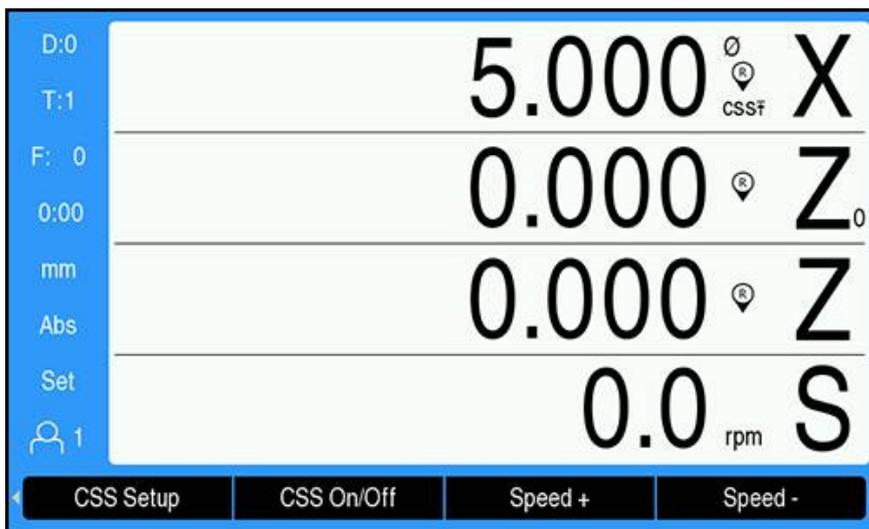
After selecting the operating **Mode** and entering its parameters in the **CSS/Direct rpm** menu, the DAC output must be enabled to begin controlling the spindle.
