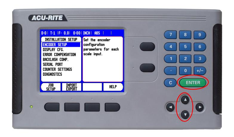
"ENCODER SETUP" should be highlighted. If it isn't, use the arrow soft keys to highlight it. Then press ENTER
