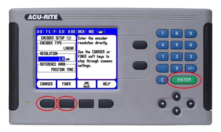
Use the "COARSER" and "FINER" soft keys to change the resolution factor until it matches what is printed on the encoder label. As you saw at the beginning, our scale is 1µm. Press ENTER to save your selection.
