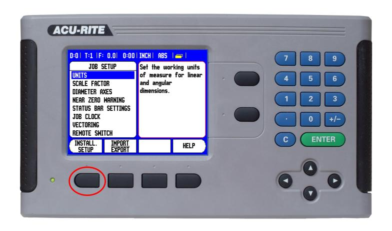
Press the "INSTALL SETUP" soft key.
