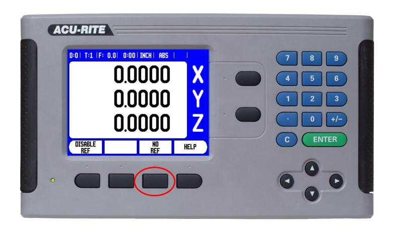
To change the resolution you don't need to reference the scale, so press the "NO REF" soft key.
