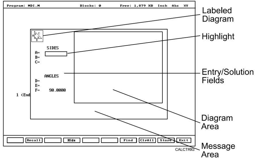
**Figure 3-3, Right Triangle Calculator Screen**
