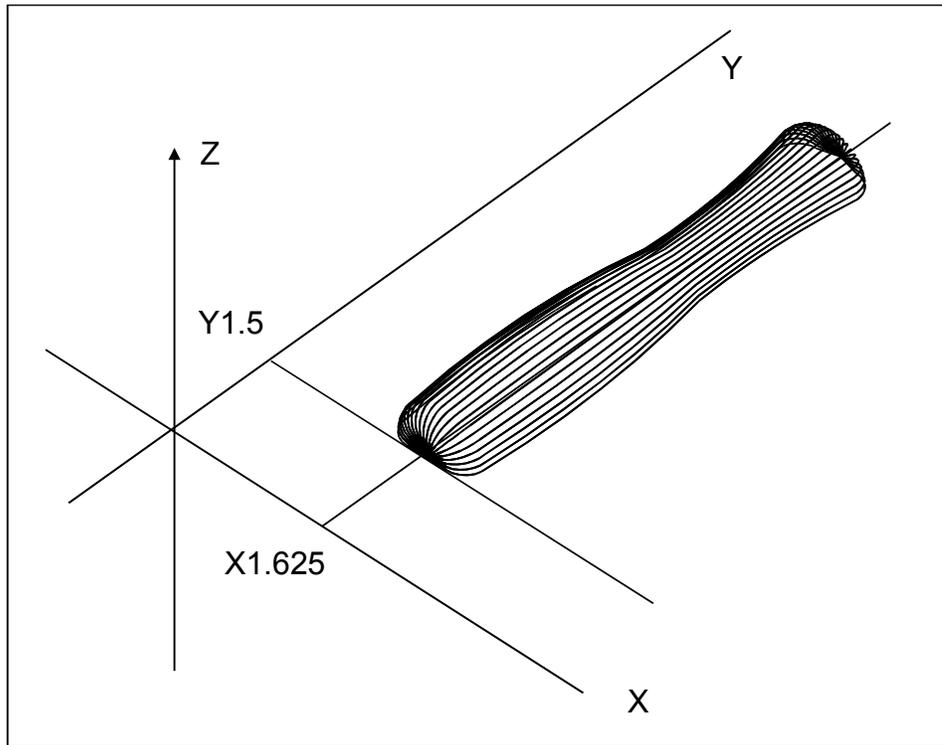
Figure 6-12, Layout for Sample Program #8 - Mold Rotation
