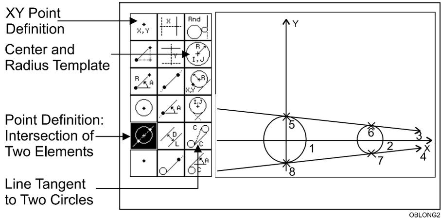
**Figure 5-11, Completed Geometry Calculator Display**
