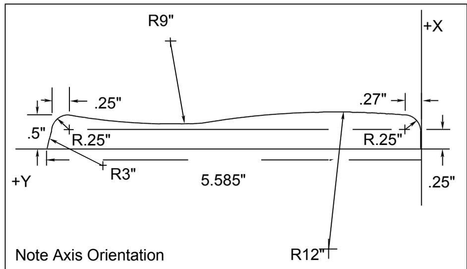
Figure 6-13, Subprogram Layout for Sample Program #8
