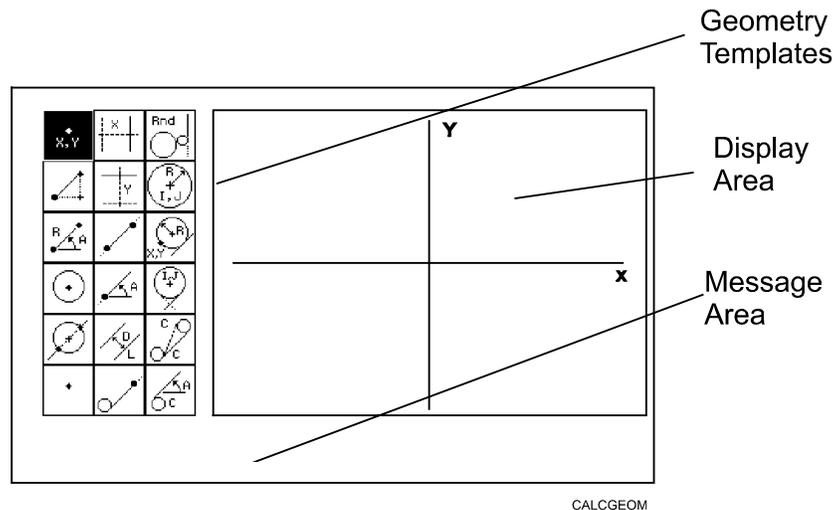
**Figure 5-4, Geometry Calculator**
