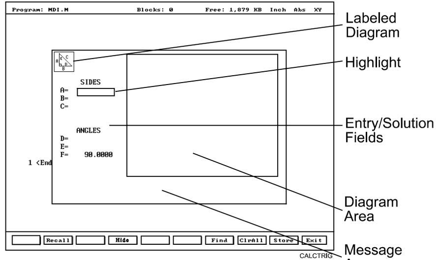
**Figure 5-3, Right Triangle Calculator Screen**
