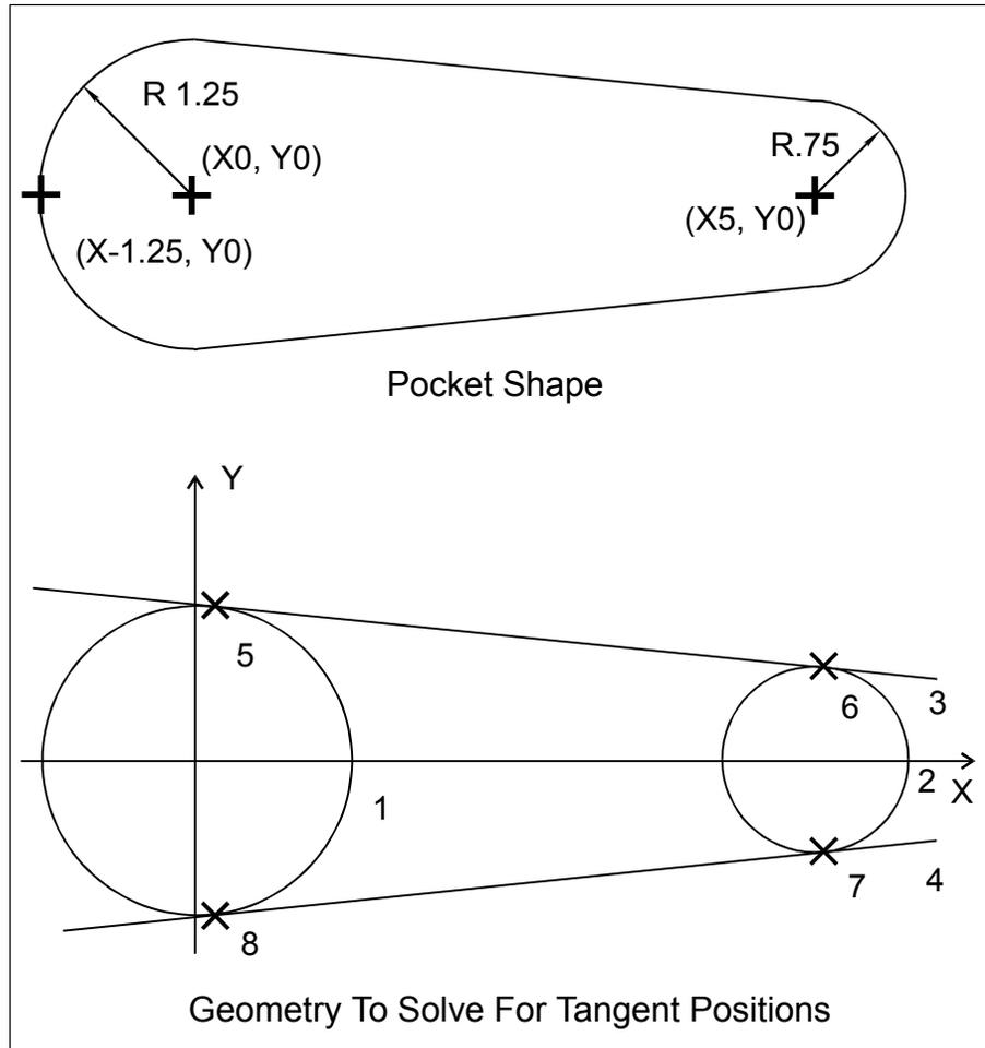
**Figure 6-3, Geometry Calculator Layout for Exercise #7**
