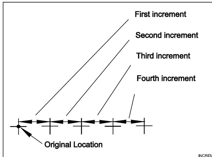
**Figure 1-3, Incremental Positioning**
