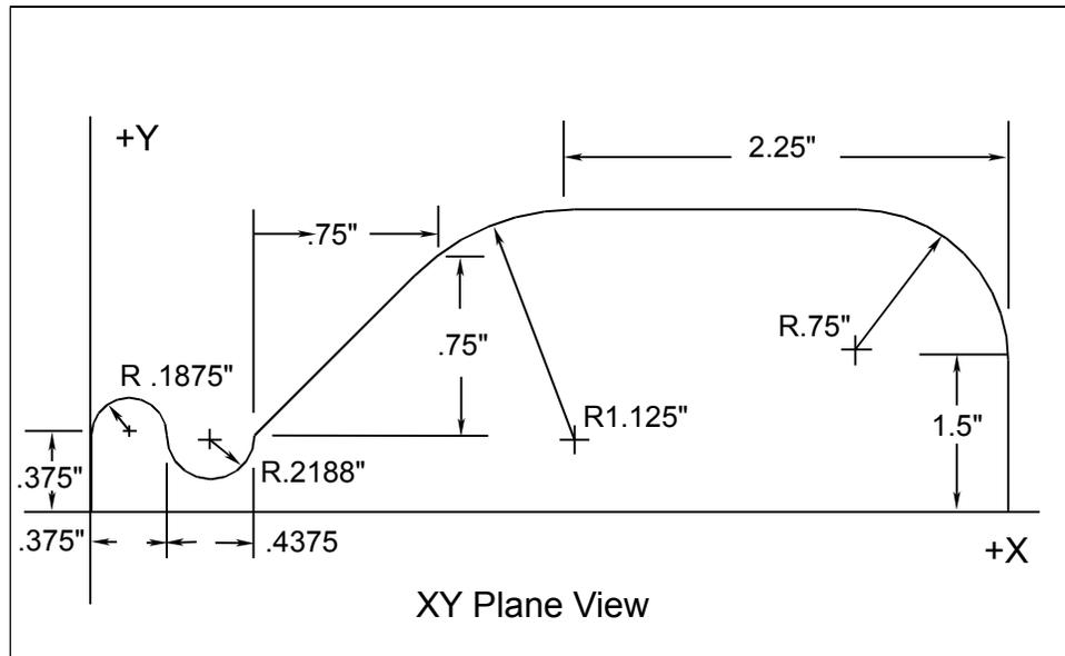
**Figure 6-11, Subprogram Layout for Sample Program #7**
