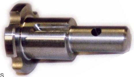
With the addition of live tooling the C-Axis gives the ability to machine key-ways, cross hole drilling, bolt hole patterns or even spiral cutting.
