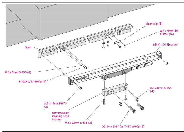
These are instructions for mounting the SENC 150 encoder to the cross feed axis with the bottom mount bracket.
