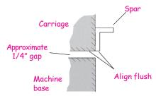
• With the cross feed at it's center of travel, hold the spar to the right side of the carriage, and position the bottom edge flush to the lower edge.
