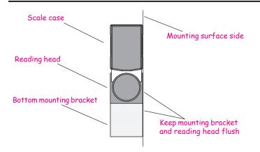
• Align the mounting surface side of the bracket flush with the reading head surface. Tighten bracket in place.
