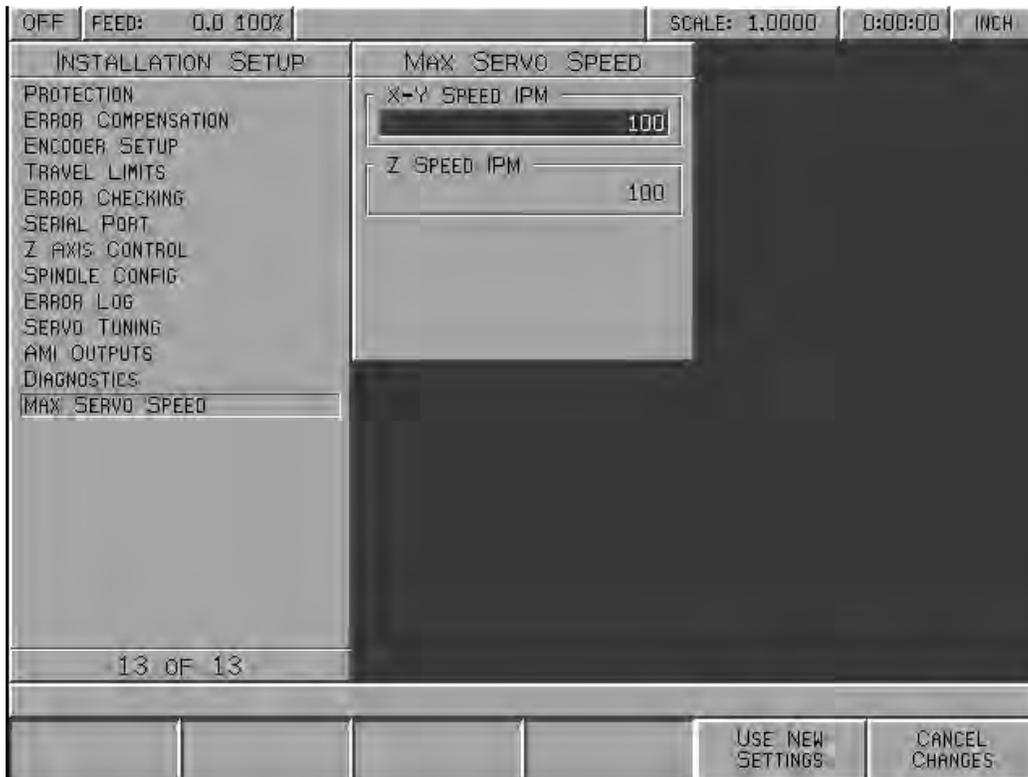
**MILLPWR** can move each axis a maximum of 100 inches per minute (IPM). This parameter allows you to establish a lower maximum speed for the X, Y, axes and/or the Z axis.
