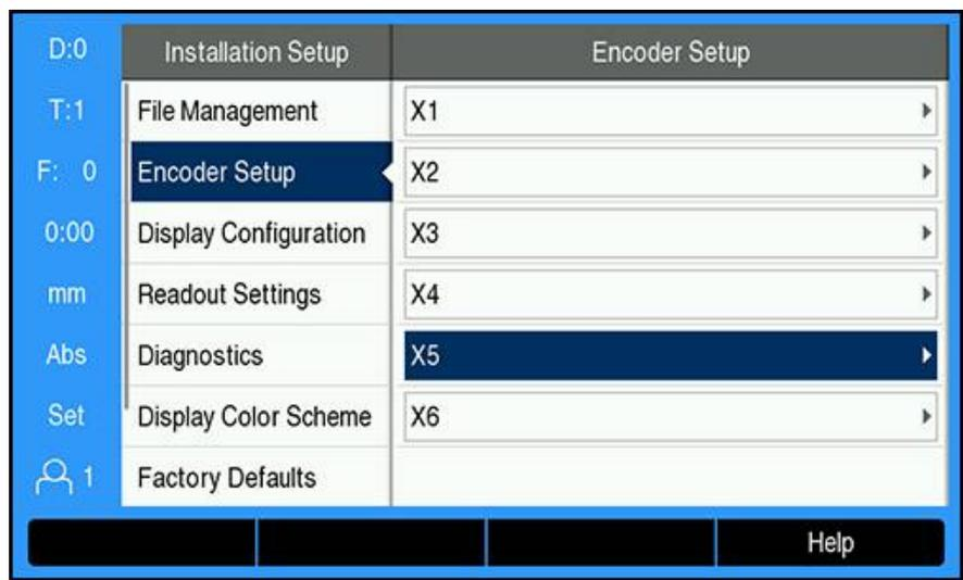
**i** The two additional encoder connections provided by the IB 2X will display as **X5** and **X6** in the **Encoder Setup** menu regardless of how many encoder connections are available on the DRO.
