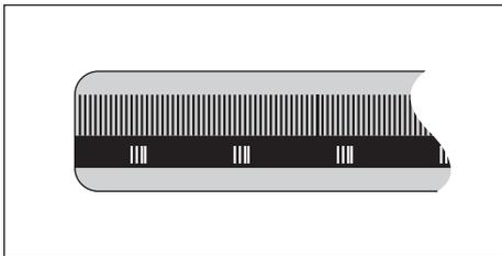
Encoders that have marks separated by a specific encryption pattern allow the product to use any two pair of marks along the length of the encoder to re-establish the prior datums. This configuration means that you only have to travel less than 20 mm anywhere along the encoder to re-establish the datums when the product is switched back on.
