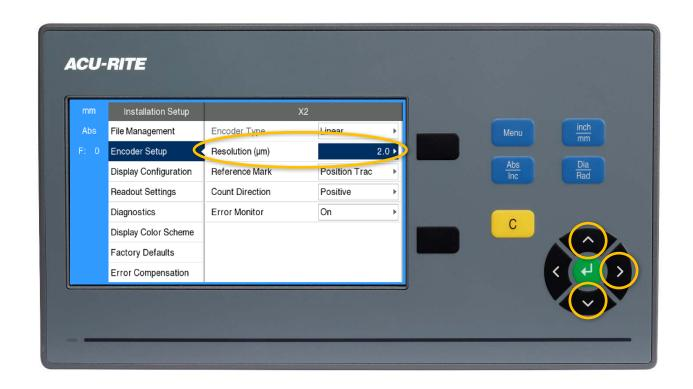
Use the up and down arrow keys to highlight the resolution that matches the encoder label, and then press enter twice.
