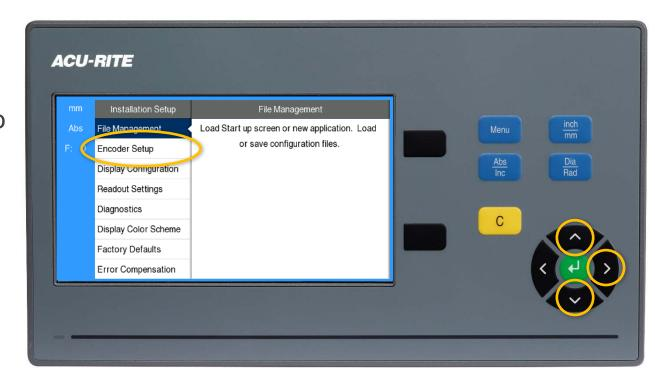
Use the up and down arrow keys to highlight the port the encoder you want to change resolution on is plugged into, and then press enter.
