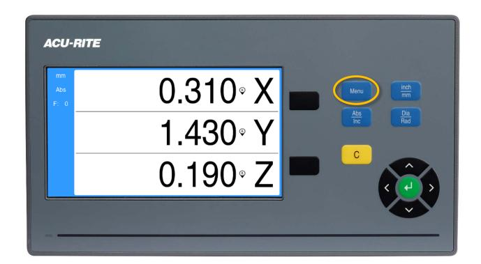
Use the up and down arrow keys to highlight the Installation Setup menu, and then press enter.
