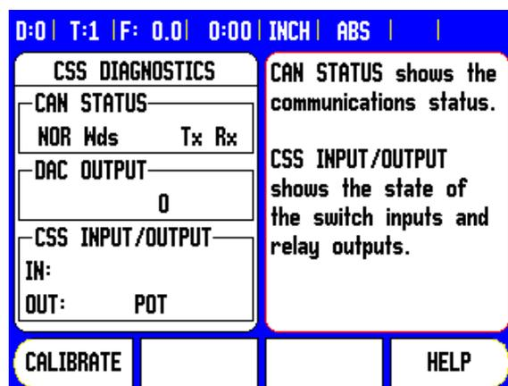
For CSS only, the MS INPUT/OUTPUT field shows the state relay outputs. The IN: field of the switching inputs is not used, and will be blank.
