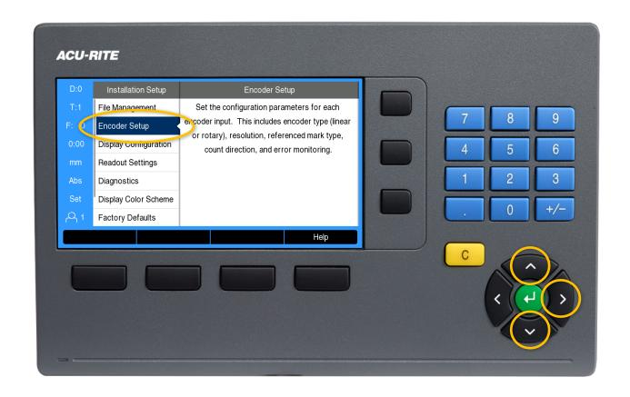
Use the up and down arrow keys to highlight the port the encoder you want to change is plugged into, and then press enter.
