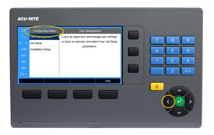
Use the up and down arrow keys to highlight the Installation Setup menu, and then press enter.
