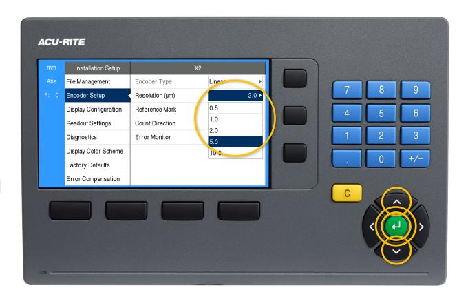
Press the left arrow key three times to get back to the DRO screen. Repeat the sequence for additional encoders as needed.
