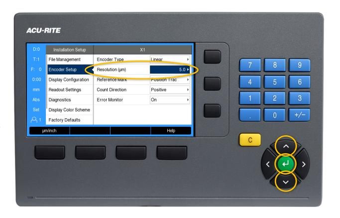
Use the up and down arrow keys to highlight the resolution that matches the value listed on the encoder label, and then press enter twice.
