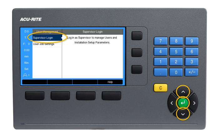
Using the number keypad to enter the passcode – 8891, then press enter.
