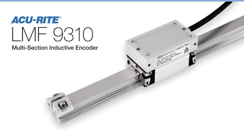
The LMF 9310 Multi-Section Inductive Encoder is a guided measuring system that uses an LMK scanning head with TTL incremental signals and an inductive measuring tape clamped on an integrated guiderail. When properly intsalled to specifications, this encoder has an Ingress Protection Rating of 67 (IP67), leaving this measurement system virtually unaffected by environmental contaminats (i.e.
