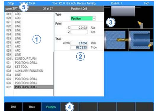
**i** Soft keys with a bar on the bottom have additional soft keys available when selected.
