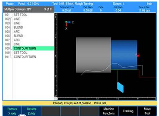
**i** If both axis soft keys are pressed, both axes will be restored sequentially in the configured order.
