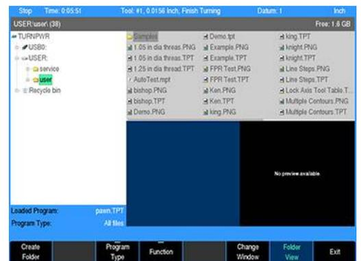
**i** It is recommended to copy programs from the USB device to the user folder and use the program from the control.
